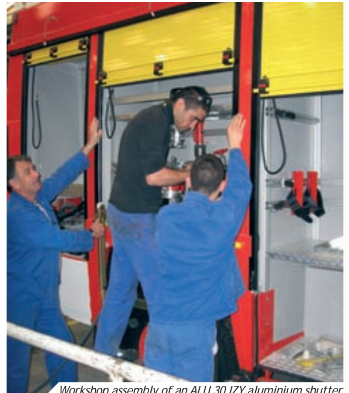
Workshop assembly of an ALU 30 IZY aluminium shutter
